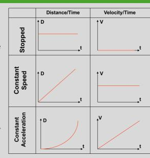
A Velocity/Time graph looks different as it plots how velocity changes over time. If velocity increases, an object is accelerating.
